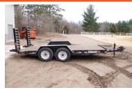
Felling FT-12 tandem axle equipment trailer-80"x16', ball hitch, stake pockets, 4' loading ramps, 12,000lb
