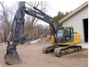
John Deere 160G hydraulic excavator-36" general purpose bucket, hydraulic thumb, JRB hydraulic coupler, 28" track pads, 620 hours, deluxe cab. s/n 1FF160GXCMF058313
