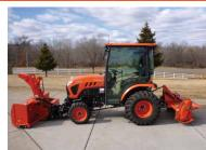
Kubota LX2610HSD compact tractor-full cab with heat and AC, includes Kubota LX 2980 front mounted snowblower with hydraulic chute, includes Land Pride RTA 1258 5' tiller, 3-point, PTO, hydrostatic foot control, joystick front controls, 3-cylinder diesel, s/n KBUB8AHCEN1C27620
